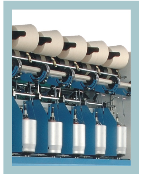
Automatic uplift mechanism Winding completed or Yarn broken, Auto lifter support lift automatic to avoid yarn grind, and also makes easy for operation.
